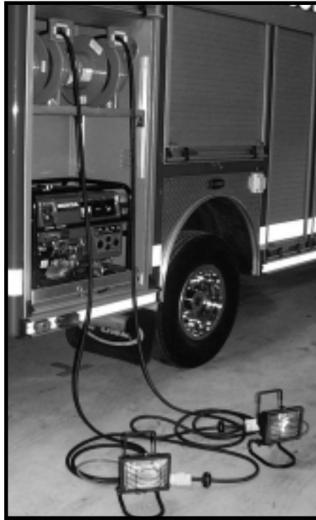
Pull out as much cable as needed to power remote lights. Spring rewind without hand cranking or coiling. Reels may be hard wired to generator or equipped with "pig tail" for greater versatility and portability.
